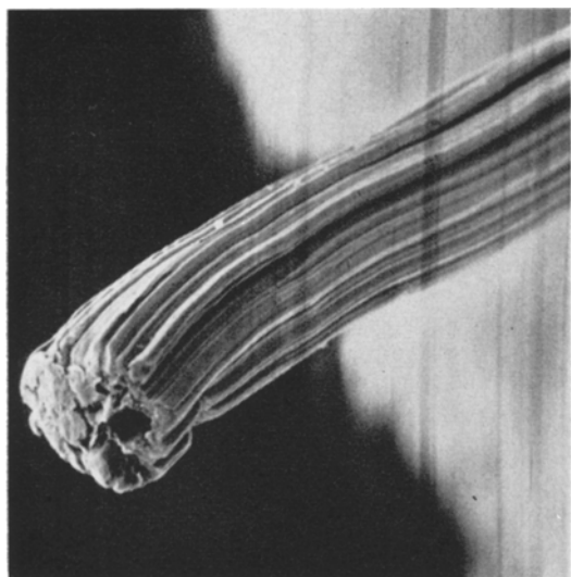
Figure 8 Base and lower section of a silver whisker which has been detached from its \alpha\text{-Ag}_2\text{S} substrate ( \times 350 ).
